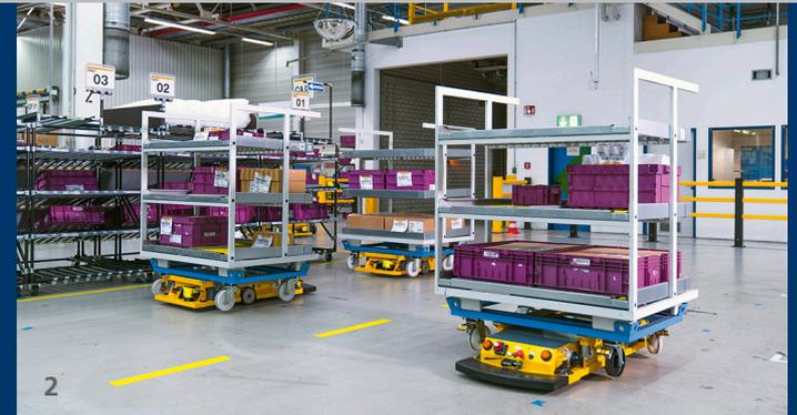
1 AGV from Bär Automation with navigation software from Fraunhofer IPA. (Source: Bär Automation GmbH)
