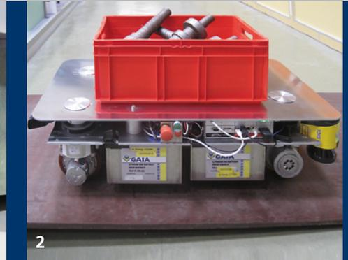
1 Built-in drive modules with steering motor.
