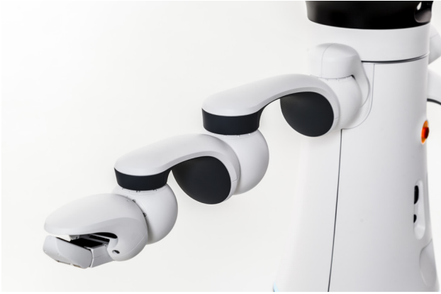
Figure 2: With its arms and one-finger-hands the robot can handle even difficult objects (Source: Fraunhofer IPA/Photo: Rainer Bez)
