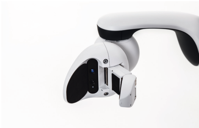
The simplicity, elegance and integrated sensors of the newly developed one-finger hand concept are impressive. (Source: Fraunhofer IPA)
