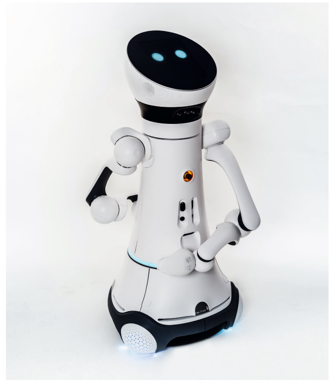
The modular construction of the Care-O-bot® 4 allows individual robot platforms to be established for a wide range of applications. This significantly reduces costs in the development of new service robot solutions. (Source: Fraunhofer IPA)
