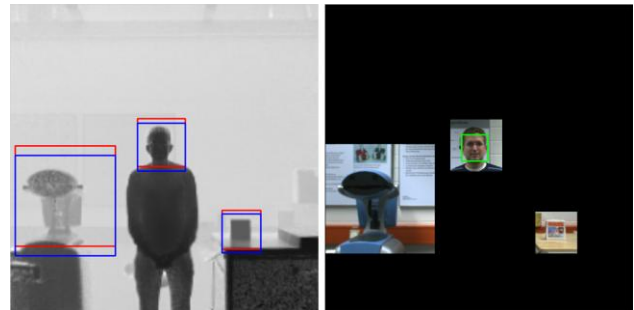
Figure 5: Detection results on the 3-D range (left) and colour image (right)
