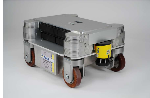
Fig. 1. Mobile base of Care-O-bot 3, without coating ( www.care-o-bot.de )
