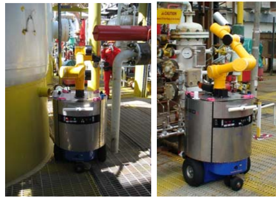
Fig. 8: Mobile inspection robot executing inspection tasks on an offshore gas platform.
