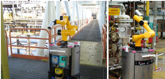
Fig. 11: Mobile inspection robot executing inspection tasks on an offshore gas platform.
