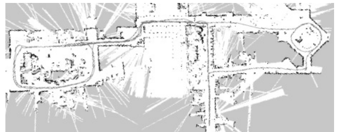
Fig. 8: Environment map and driven path for navigation tests (black: detected obstacles, white: free space, grey: unknown).
