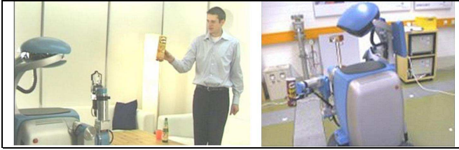
Fig. 4: Illustration of the basic components for the interactive and active object learning scenarios. In the interactive mode the human holds the object; in the active mode the robot holds it. In both cases the rough location of the region surrounding the object in 3D space is available (see text). The object is then rotated in order to produce sample appearances.
