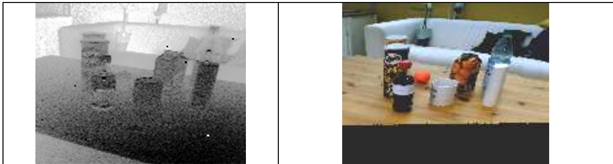
Figure 8: Left: The range image (with normalized histogram for illustration). Right: The color values for pixels in the range image generated with the direct calibration that uses eleven parameters. The black banner at the bottom is caused through the mechanical setting of the sensors.
