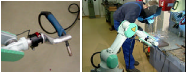
Figure 7. Prototype of robot assistance for manual arc welding
