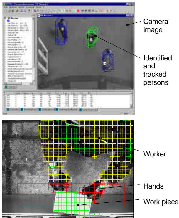
Figure 5: Monitoring the robot assistant's workspace by visual sensors from the ceiling (above) and the workbench (below), courtesy Fraunhofer IPK and Fraunhofer IWU.
